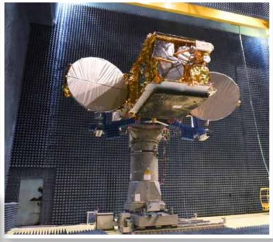
GSAT-19 maintains the satellite's orientation with the help of momentum wheels, magnetic torquers and thrusters. The satellite's propulsion system consists of a 440 N Liquid Apogee Motor (LAM) and eight 10 N and eight 22 N Chemical thrusters using liquid propellants for initial orbit raising and station keeping.
