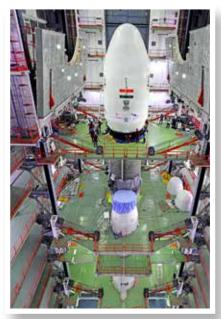
This fourth generation launch vehicle is a three stage vehicle with two Solid Strap-on Motors S200, a Core Liquid Booster L110 and a Cryogenic Upper Stage C25. The vehicle is configured with a 5 m Ogive Payload Fairing (OPLF) and slanted strap-on nose cone to provide aerodynamic robustness.
